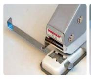
Adjust the paper side lay on the TC 20 to the correct calendar width.
